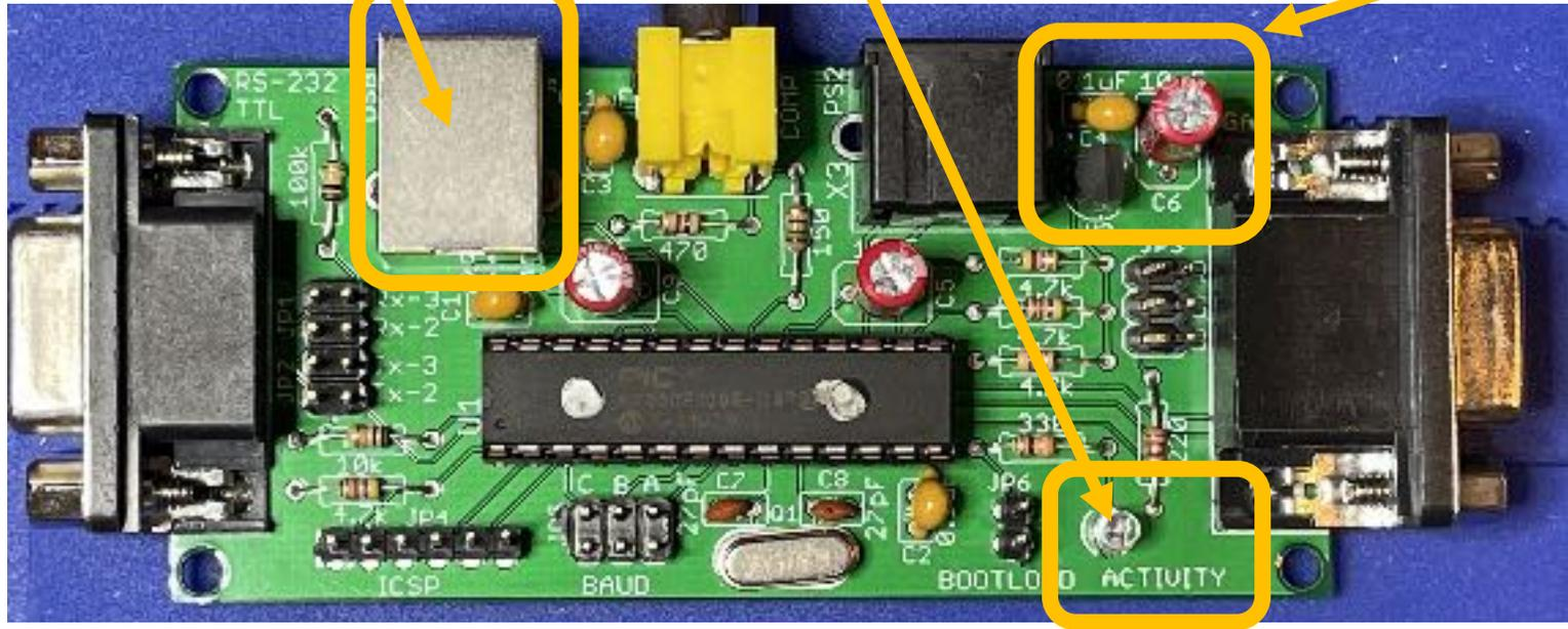
*YOU CAN ALSO METER THE LED (POSITIVE ON THE BOTTOM)*
