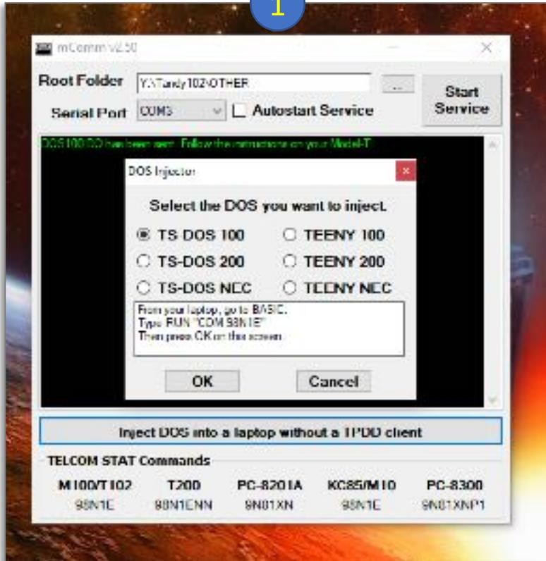
INJECT TS-DOS (OR TEENY) USING MCOMM V2.50 OR WHATEVER YOU PREFER. YOU NEED A WAY TO LOAD THE CONFIG FILE ONTO THE MODEL T.
