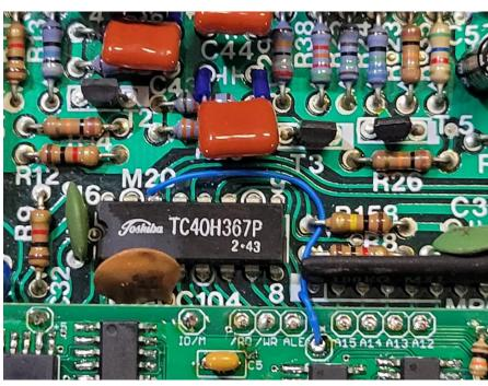
Cut track as indicated to disconnect the A\* signal from the SRAM subsystem.
