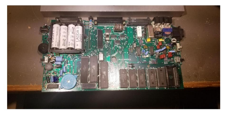
Here we have removed the main PCB from the case. Also, removed the ribbon cables carefully.
