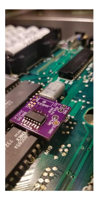
Now that the clock divider is installed, you must connect the new 2.5MHz clock to the system clock signal.
