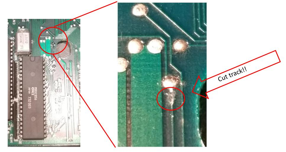
Pin 37 of the CPU drives the system clock signal. That must be disconnected. One way is to cut the clock track at the indicated location.
